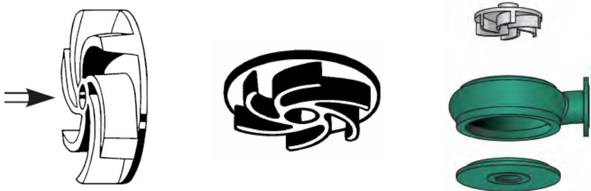
Abbildung 4-26: Freistromrad (ATV-DVWK-A 134, 2000; JABERG, 2003; WILO, 2008)
